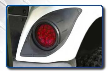
Install new tail light using supplied hardware. \*Repeat process on opposite side
