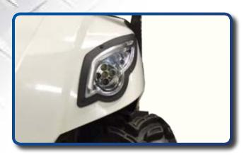
Mount headlight through the cutout using supplied fasteners.
