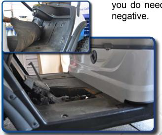
Remove all plastic rivets from floor mat. Retain hardware. Remove floor mat.
