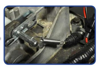
Mount indicator assembly using clamps provided and tighten. Run indicator harness along steering column and insert harness through dash.
