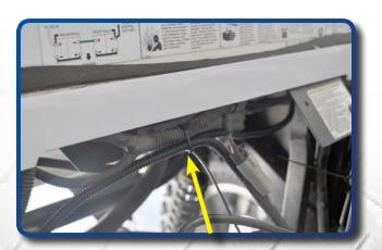
Tie the wiring harness to the main harness at the back of the battery compartment as shown.
