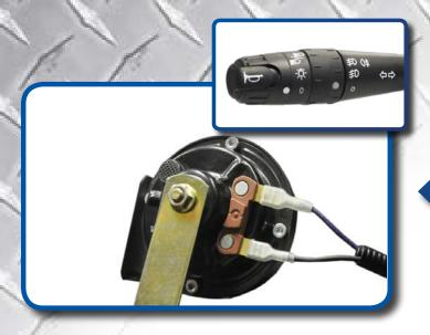
Attach horn to purple and black female spade connectors and secure horn to metal frame under front cowl using supplied hardware.
