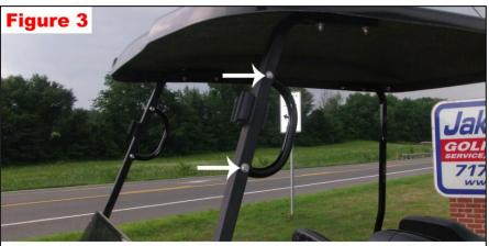
Mount brackets to the inside of the roof struts as shown with supplied hardware. Club Car/Yamaha 1/4 x 1 3/4, EZGO 1/4 x 1 1/4
