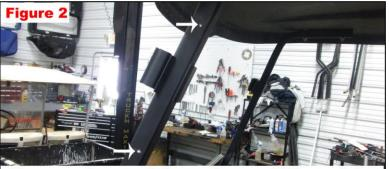
Use a center punch to mark your drilling points. Using a 5/16 drill bit, drill through the roof struts.
