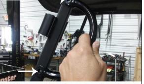
Hold in desired location and mark roof struts
