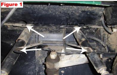
Enlarge the four stock shock shield cover mounting holes to 3/8"
