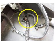
13. Secure the middle portion of the harness to the underbody of the cart. Use a 1/4" drill and drill (5) holes in the plastic underbody.
