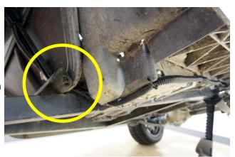
11. Locate the rectangular hole in the bottom of the splash guard. Use a utility knife to enlarge the hole enough to fit the harness.
