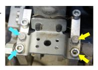
Slide the LGT-161 brake switch bracket under the original stop bracket on the driver side. The wires should face the rear. Align the slots with the holes in the brake assembly. Reinstall the <u>Original</u> <u>Hardware</u>. Do not tighten.
