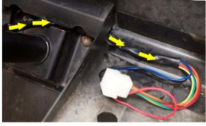
5. Connect the included flasher relay to the turn signal switch wiring harness.
