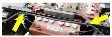
Disconnect the pushpull switch at the 4-pin connector and the jumper from the 9-pin connector.
