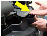
3. Install the headlight bumper using the <u>Original Bumper Hardware</u>. Keep the original nuts and washers in place between the bumper
