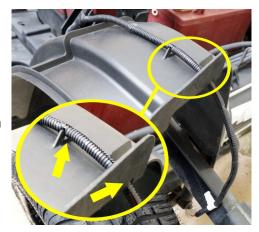
8. Secure the passenger taillight cable to the rail of the frame with cable ties using the pre-drilled holes in the frame.
