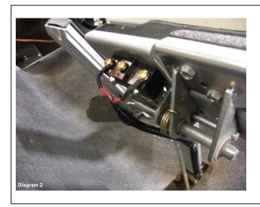
**Step 2:** Install the micro switch with the longer of the two leads onto the reverse side of the brake pedal (see diagram 2) using the included hardware.
