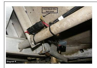
**Step 4:** Attach the two pin connector from the LGT-641 Brake Switch Kit to the two pin connector from the LGT-695 Wire Harness (see diagram 4). Secure all loose wires being certain that no wires are crimped or pinched.
