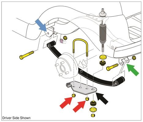
15. Place a lift block on top of the axle, in the perch. When orientated correctly, the lift block will slope downwards toward the front of the cart.
