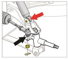
12. Remove the (3) bolts in the steering rack. Retain hardware.
