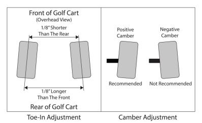
2. Adjust the toe by loosening the jam nut on the tie rod. Lengthen or shorten the tie rod by turning the hex shaped rod adjustment. Adjustments should be made evenly on both sides.
