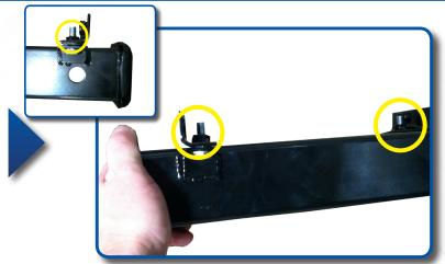
Using 8x40mm hardware, attach trailer hitch to footrest as shown.
